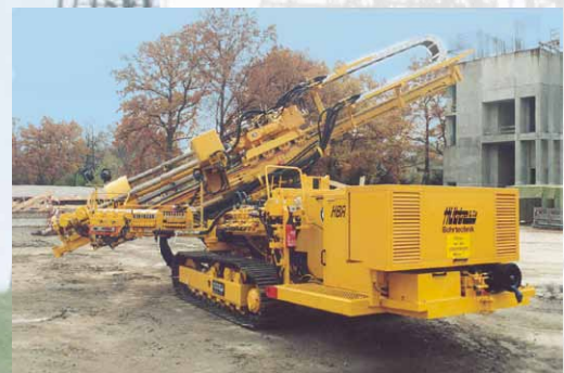
Mobile deep drill rigs, Hütte & Co.
